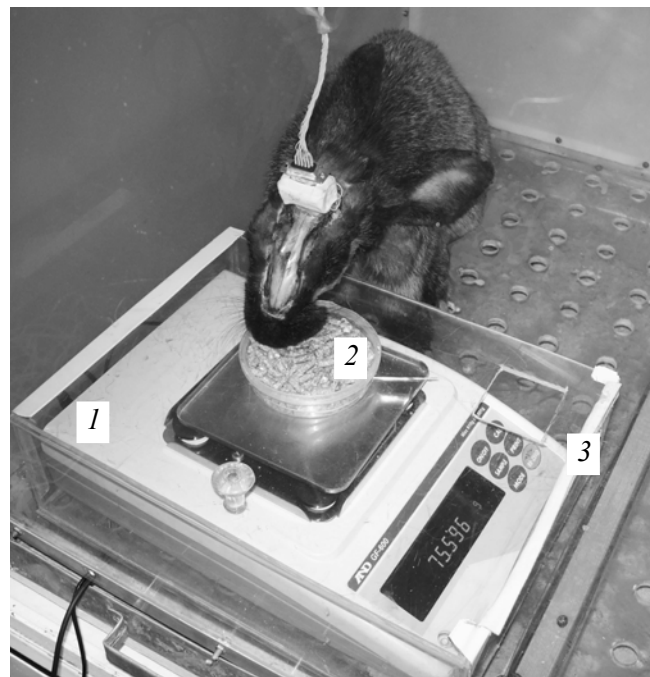
Fig. 1. Recording of food-procuring behavior of a rabbit under conditions of free access to food in a rack placed on a platform of an electronic balance. 1) GF-600 electronic balance; 2) food rack with pelleted food; 3) balance cover.
